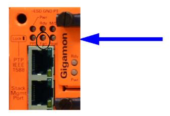
Figure 5 Fan LED Location on GigaVUE-HC2 Front
