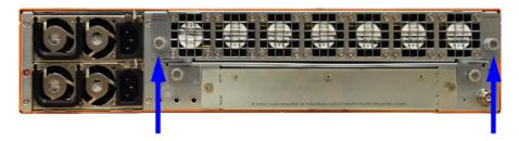
Figure 6 Fan Tray Screw Location on GigaVUE-HC2 Rear
