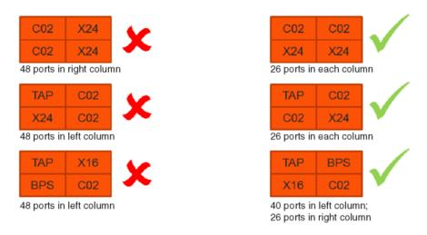
Figure 7 Module Placement of PRT-HC0-CO2, 100G Mode
