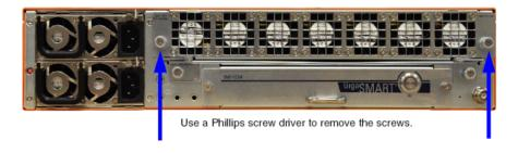
4. Remove two lower screws as shown in the following figure.
