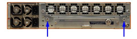
5. Turn both latches outward as shown in the following figure to release the control card from the chassis.
