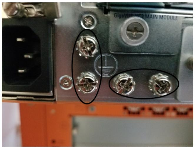
**Figure 1** Grounding Points for Ground Screws (GigaVUE-HC2 Shown)
