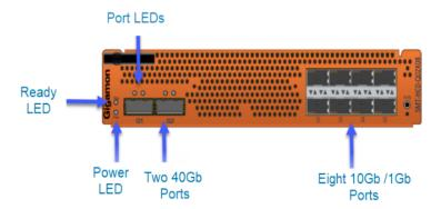
Figure 18 GigaSMART Front Module
