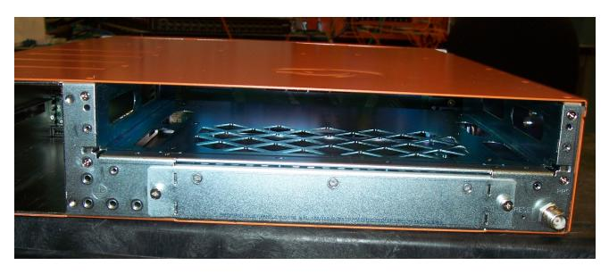
**Figure 9** Back of Node Shows Opening for Control Card
