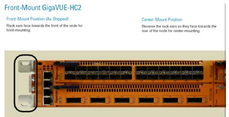
**Figure 2** Rack Ears for Front Mount (Reverse Rack Ears for Center Mount)
